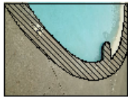
SW EDGE OF POOL AREA OF CONCRETE REMOVAL
