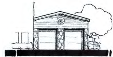
Figure 6-5. Only single entry doors are allowed if the garage is front loaded and facing the street.
